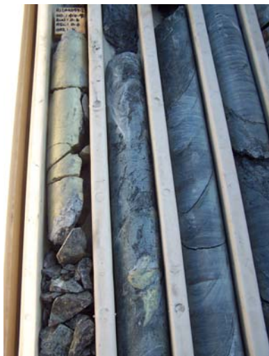
Plate 1: Copper sulphides in sheared sediments in Rover 12 drillhole R12ARD59-2.
