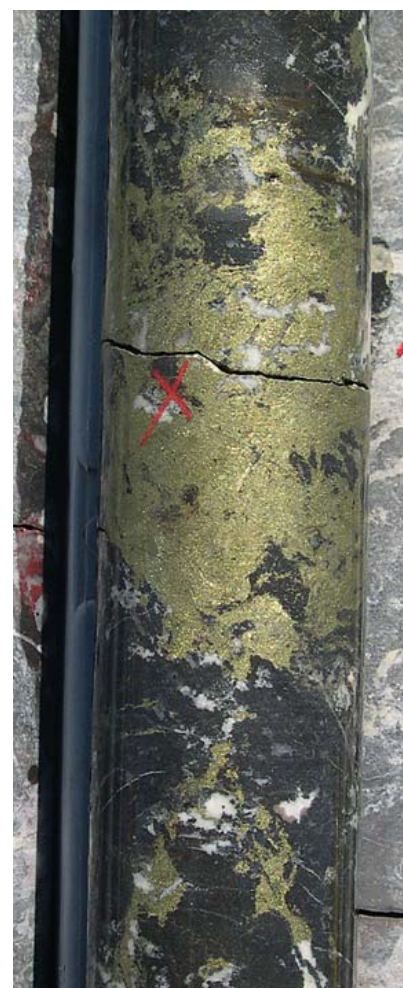
Chalcopyrite (copper sulphide) in a black magnetite rich matrix in hole R4ARD21. Core diameter ~51mm.
